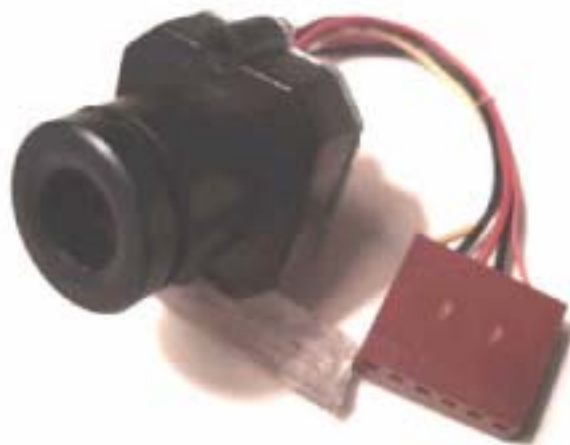
Figure 10 Project Camera Modified with Connector and Base Mounting
