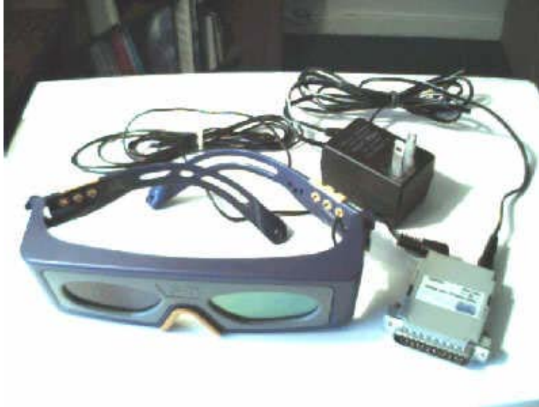
Figure 48 Mcnaughton 3D-Spex shutter glasses
