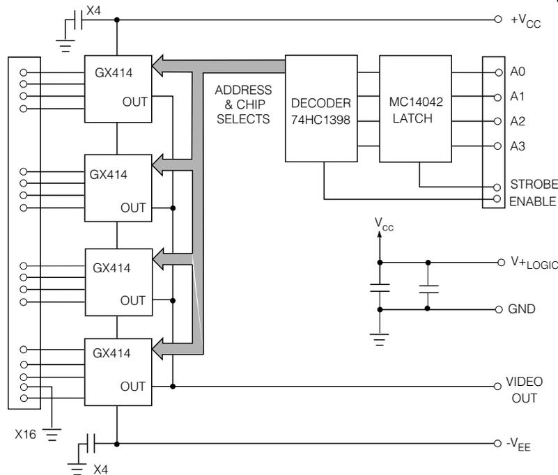
Fig. 1 Circuit Diagram of the 16x1 Multiplexer
