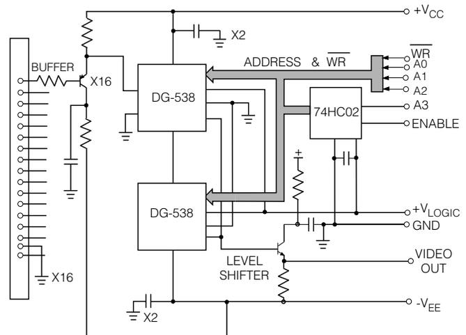
Fig. 3 Circuit Diagram of a DG-538 16x1 Multiplexer
