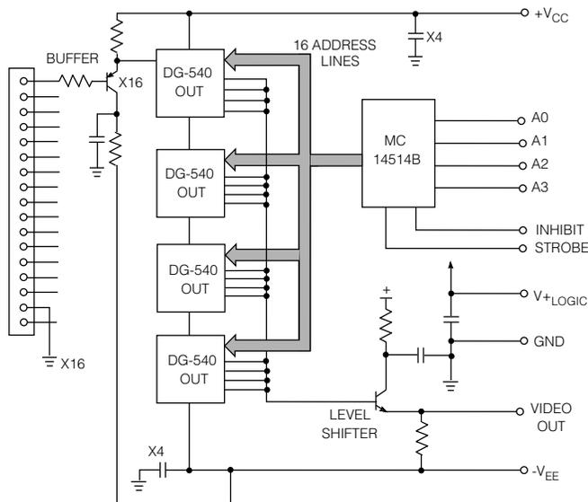
Fig. 4 Circuit Diagram of a DG-540 16x1 Multiplexer
