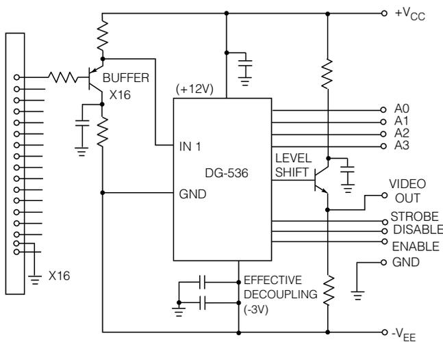
Fig. 2 Circuit Diagram of the DG-536 16x1 Multiplexer
